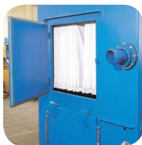
The filtering system is composed of a primary, fabric, pocket filter and safety cartridge is class M; also available in the absolute version certified for the suction of noxious dust such as asbestos (class H).
